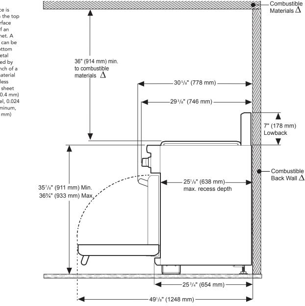
$\Delta$  As defined in the "National Fuel Gas Code" (ANSI Z223.1, Current Edition). Clearances from non-combustible materials are not part of the ANSI Z21.1 scope and are not certified by CSA. Clearances of less than 6" (152 mm) must be approved by the local codes and/or by the local authority having jurisdiction.
