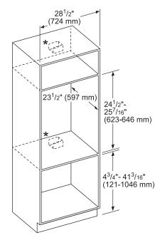
\* For single ovens installed into a wall cabinet, the junction box may be located above, beneath left or right of the unit within range of the power cord.
