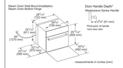
Steam Oven Wall Mount Installation Dimensions for Under-Counter Installation
