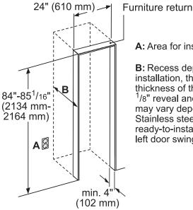
A: Area for installation of power connection.
