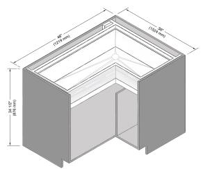
If your cabinet(s) have been built to accomodate your Galley, proceed to step one. If you are joining two or more cabinets together to house the Galley, you will need to trim the bulkheads to create an 11" clearance for the basin.
