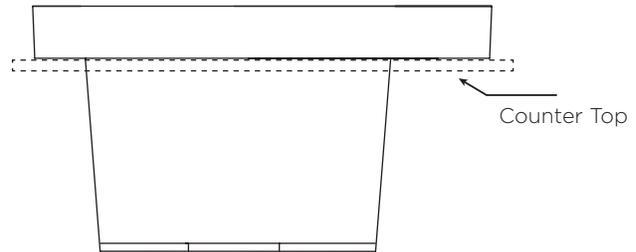
**STEP 2:** Place a generous portion of plumbers' putty under drain cap and insert whole drain body inside the bowl and through the countertop.
