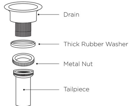
**STEP 3:** From under the drain, insert the thick rubber washer and screw on and tighten the metal nut. Remove excess plumbers' putty
