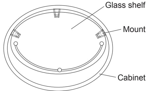
**Step 2 :** Unscrew flat head setscrews in glass shelf mounts (3) located inside cabinet
