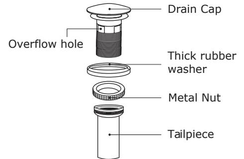
**Step 5 :** From under the drain, insert the thick rubber washer and screw on and tighten the metal nut. Remove excess plumbers' putty.
