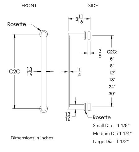
**Installation Notes**: Center to center hole drilling dimension are same as mentioned in column. <u>Diameter of glass hole for installation is 1/2".</u>
