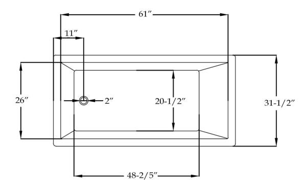
Weight (empty): 429 lbs Weight (filled): 957 lbs Capacity: 63 gal Water depth: 16-1/2"
