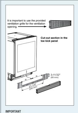
The cut-out section in the toe kick panel must be centered in relation to the appliance and in the uppermost part of the toe kick.
