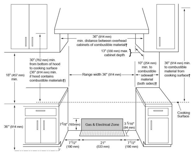
† as defined in the "National Fuel Gas Code" (ANSI Z223.1, Current Edition). Clearances from non-combustible materials are not part of the ANSI Z21.1 scope and are not certified by CSA. Clearances of less than 12" (305 mm) must be approved by the local codes and/or by the local authority having jurisdiction.
