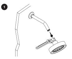
Using an adjustable wrench, remove the showerhead.
