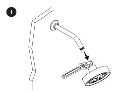
Using an adjustable wrench, remove the showerhead.
