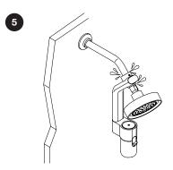
□ Turn ON the water and check for leaks.
