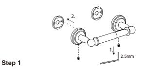
Loosen the set screw on the accessory and remove the backing plate. Position the accessory against the wall and mark outline with pencil.
