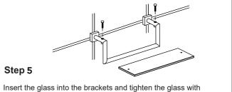
Insert the glass into the brackets and tighten the glass with set screws.
