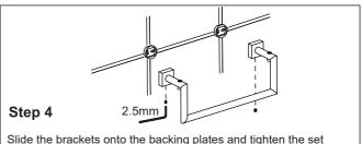
Slide the brackets onto the backing plates and tighten the set screws using Allen key provided.
