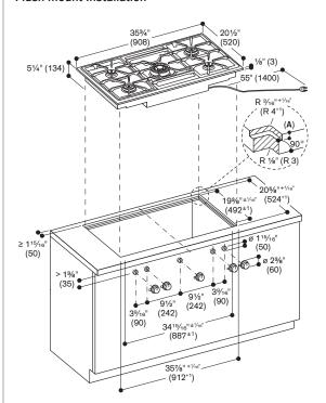
Minimum countertop thickness 1 3/16" (30 mm) for flush installation.
