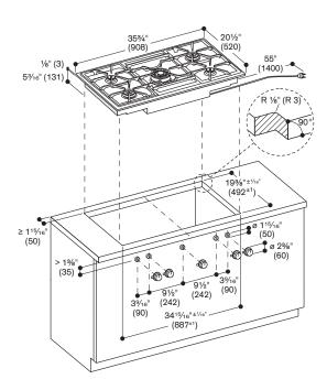
Minimum countertop thickness 3/4" (20 mm) for surface mounted installation.
