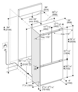
The door face dimensions are designed for a maximum gap of  $1\!/\!\!s$  " (3 mm).
