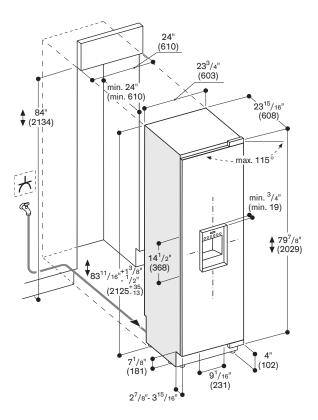
The door face dimensions are designed for a maximum gap of 1/6" (3 mm).
