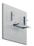
5 Slip connect the Shell to the upper brackets thru the eyelets.
