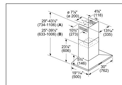
Installation height above cooking surface: 30"-36" (762 mm-914 mm) to Electric 30"-36" (762 mm-914 mm) to Gas
